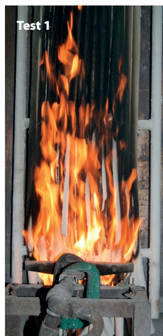
Coated cables exposed to 20kW gas burner during test
