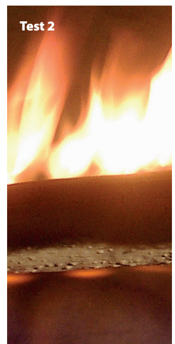
High voltage cable exposed to 700°C flame
